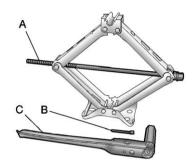
The tools you will need to change a tire include the jack (A), extension and protection guide (B), and wheel wrench (C).
